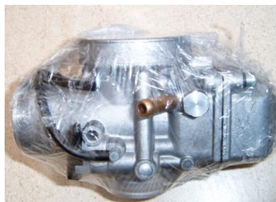
Now at this stage in an effort to maintain carb cleanliness and not undo this careful preparation, I always wrap my re-built carbs in cling film and then a soft clean rag to protect against knocks, only refitting to the engine on race day. This practice I find also helps to eliminate any condensation issues with warm carbs then stored in a cold garage. That said a good carb should always be kept warm under your pillow!
